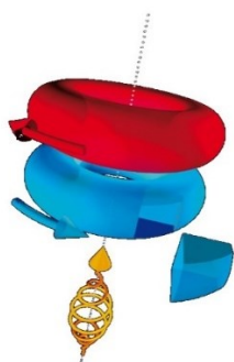
Figure 1. Illustration of a circularly polarized laser pulse (orange) that selectively liberates electrons with a magnetic quantum number of m = -1 (blue) compared to electrons with m = +1 (red). Here, in a semi-classical picture, the m = -1 electrons are counter-rotating with respect to the electric field of the circularly polarized laser pulse.
