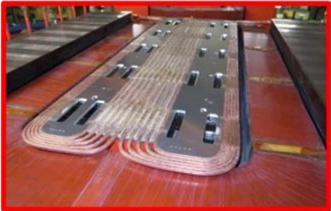
10 trim coils for precise isochronous field
